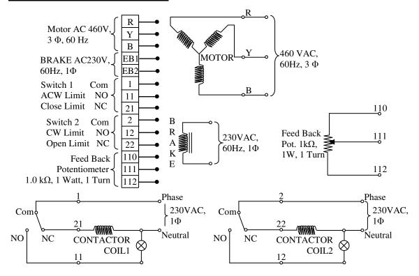
**Note:** The Motor & Electro-magnetic Brake should be powered simultaneously at their rated values. The motor can not run with the brake in off condition. For single phase connections, please call.
